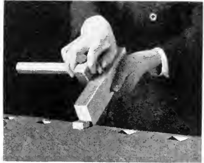
Fig. 5. The Marking Gauge in Use.
